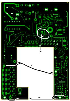
Note: The small HT-7-1 microphone preamp board connects to the other end of the cable that is shown at "C" above. There is a section of bare wire attached to the crystal that you can connect to the braid and then cover with heat shrink tubing.
