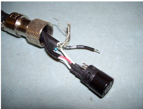
Place heatshrink tubing over the black wire and apply heat
