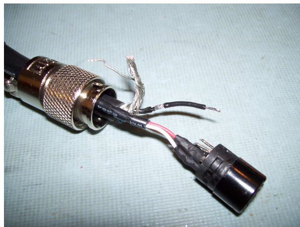
Unsolder pin 7 from the connector and cut the shield wire off of it
