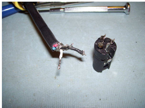
Unsolder all wires
