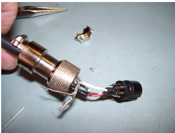
Slide the shell & plastic ring away from the 8-pin connector
