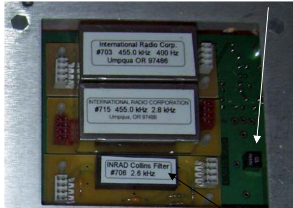
455kHz IF: Collins mechanical filter in slot 2
