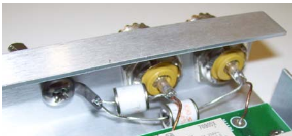
Gas discharge tube mounting
