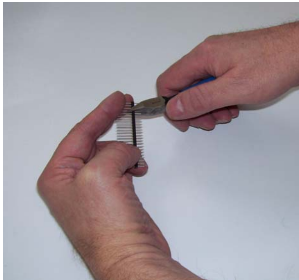
Detail E1. Cutting 36-pin connector into 12 4-pin connectors
