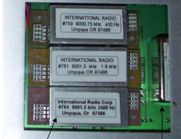
Photo K1: Typical filter installation
