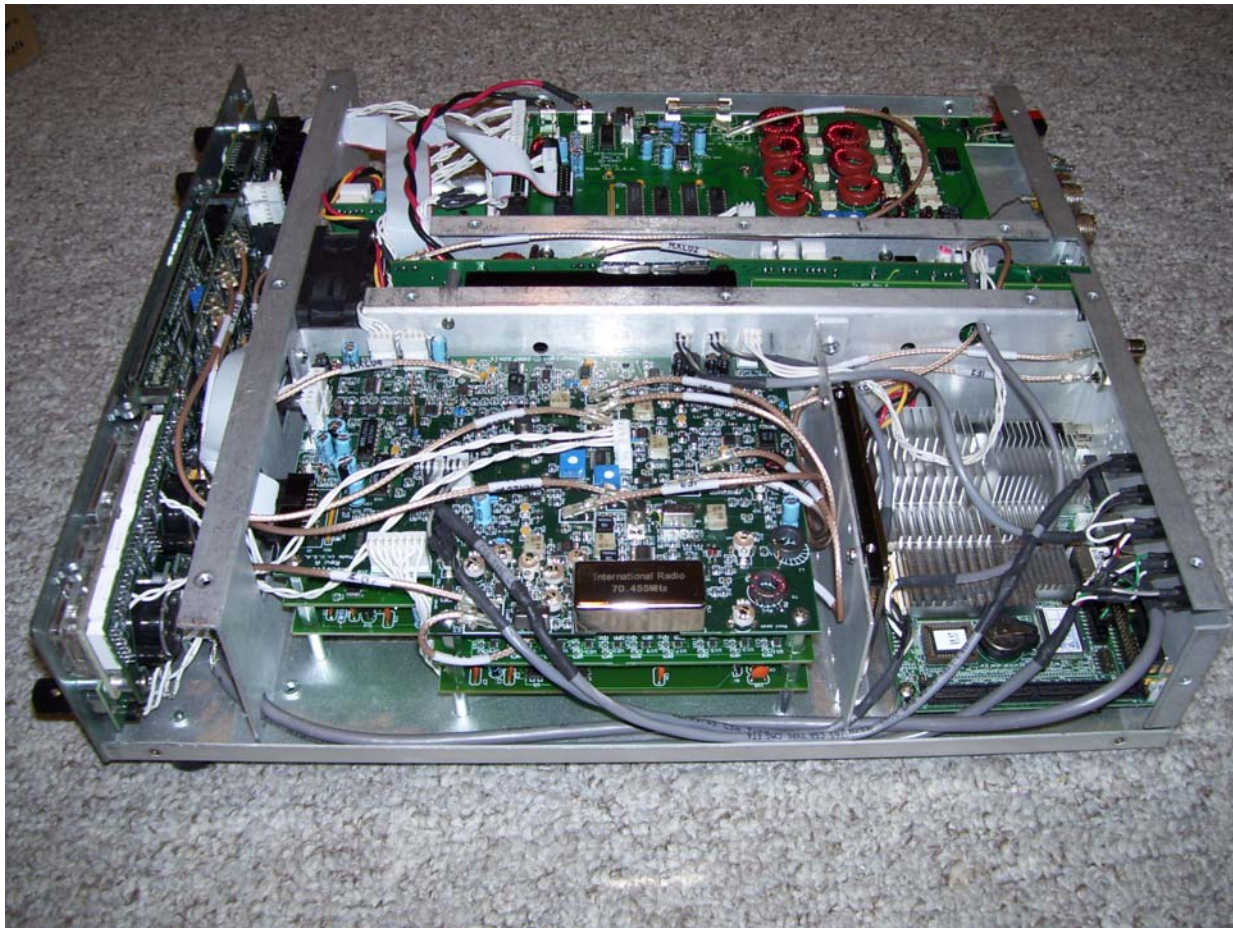
Pictorial 6. Completed unit showing cable dress from controller
