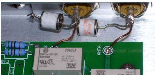
Detail 5. Gas discharge tubes
